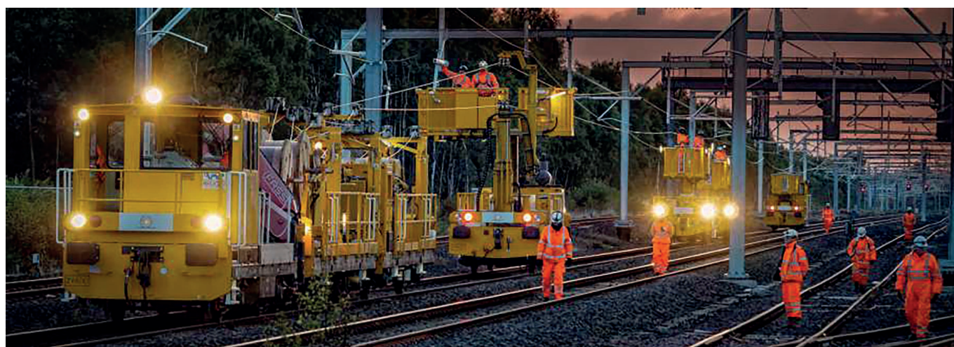
Fig 23. A typical contractor owned wiring 'train'
