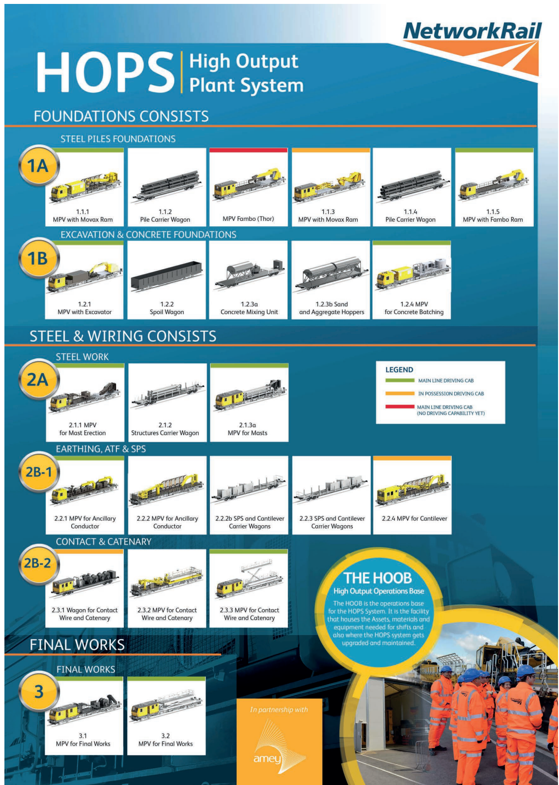
Fig. 19 The High Output Plant System (HOPS)
